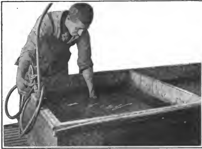
Stage 10—Giving the final test for leaks in the finished radiator
